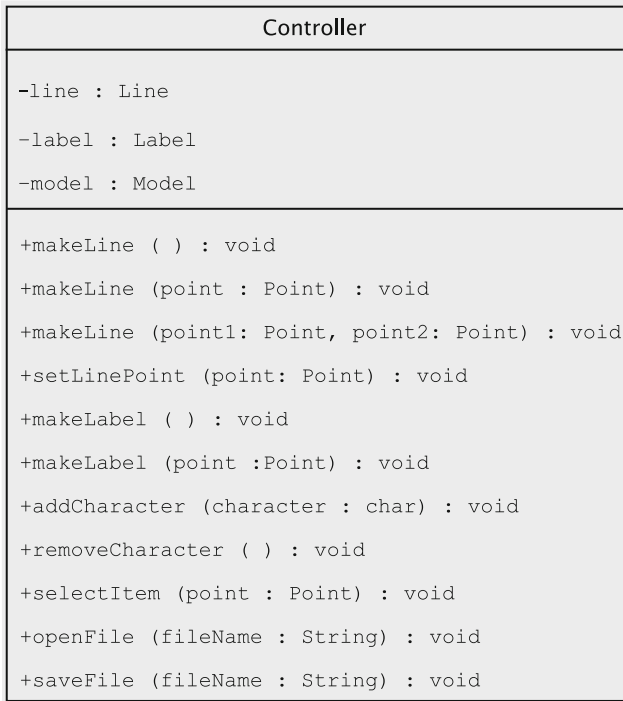
Fig. 11.12 Controller class diagram
