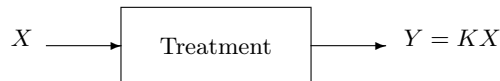
Fig. 8.1. Treatment system for spill water; X : concentration of pollutant before treatment; Y : concentration of pollutant after treatment; K : efficiency of treatment.
