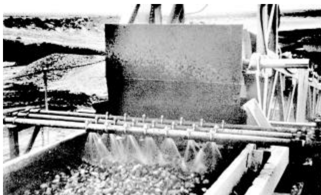
Fig. 2.5.5—Coarse aggregate rewashing
