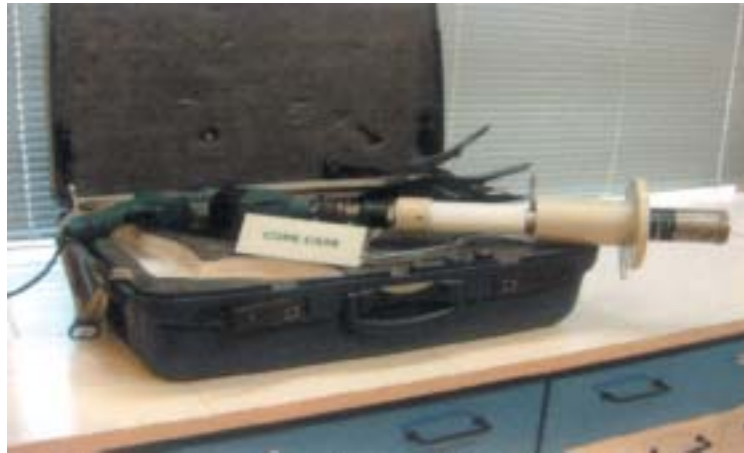
A view of rotary core cutting drill with necessary arrangement, ready to extract 50 mm dia core.
