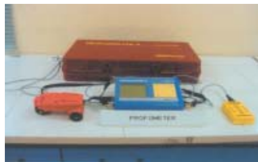
A view of Profometer with attached Scanner to locate the reinforcements and to determine spacing, diameter and concrete cover.
