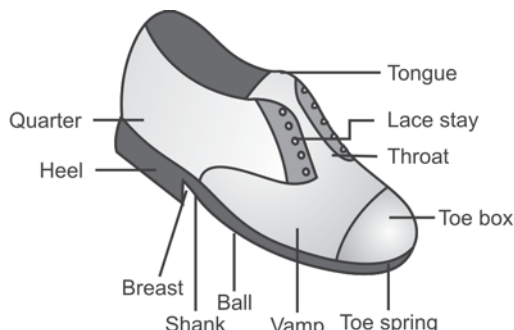
Fig. 29.1: Parts of normal shoe
