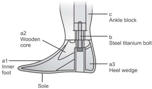
Fig. 7.9: Solid ankle flexible keel foot
