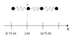
**Fig. 18.5** (Atomistic model for longitudinal waves) A set of mass points m is connected by springs with stiffness K. The elongation of mass point number j from its equilibrium position  $x_j = j\Delta x$  is  $\xi_j$ . The equations of motion  $m\ddot{\xi}_j = -K(\xi_j - \xi_{j-1}) - K(\xi_j - \xi_{j+1})$  coincide with (18.20) with a velocity of  $c = \Delta x \sqrt{\frac{k\Delta x}{m}}$
