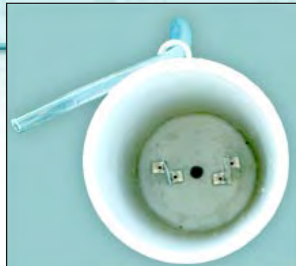
Looking down into the electrolyzer, with the electrodes in place. The height gauge tube is visible at the upper left. It is connected to the black barb splicer, visible in the center.
