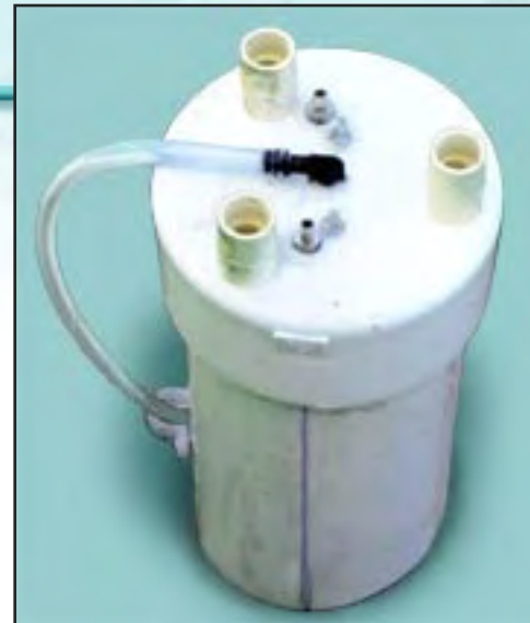
The electrolyzer upside-down, without the top cap
