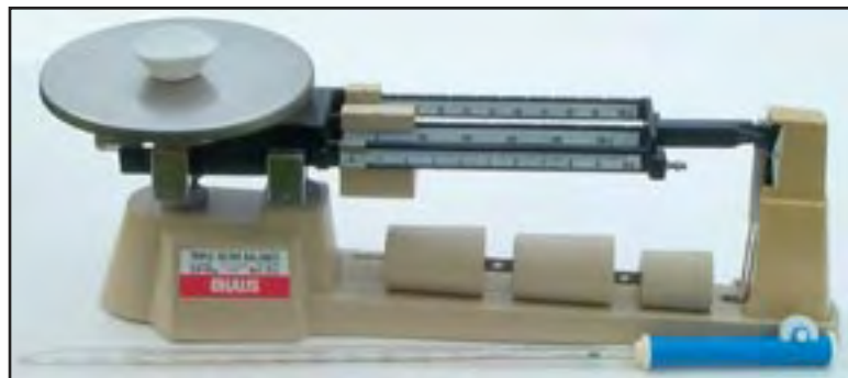
Scale with glassine “candy cup” for weighing chemicals. Pipette with pump is in the foreground.
