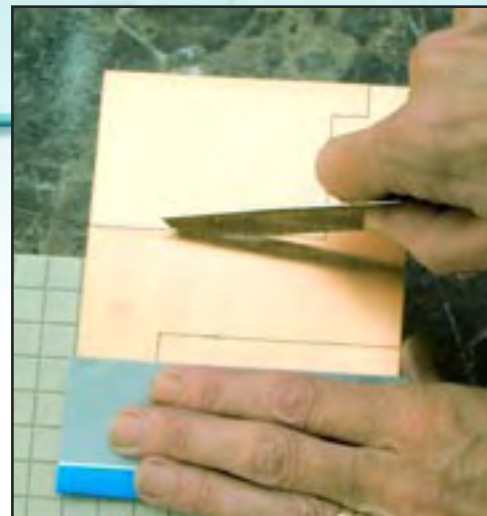
Cutting the end plates from the circuit board
