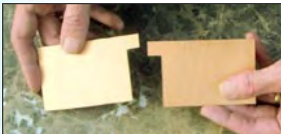
The two end plates, ready to drill
