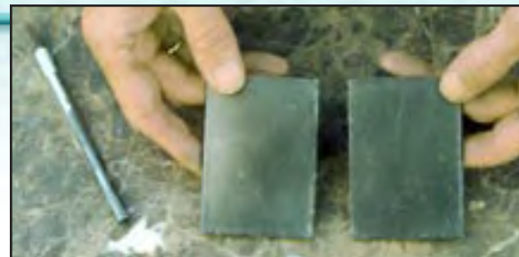
Two plates cut from graphite foil
