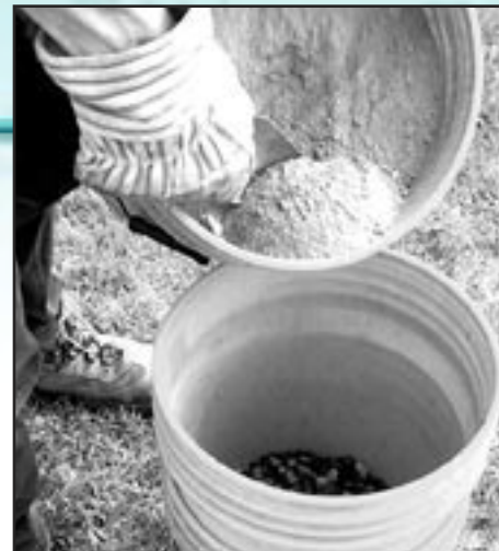
Add the ashes to the filter bucket
