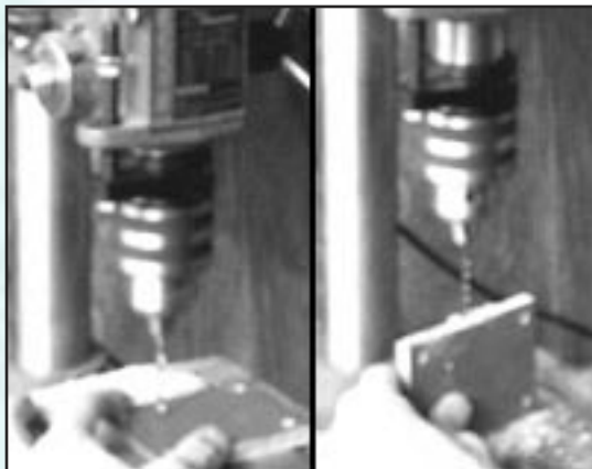
Drilling fiberglass end plates
