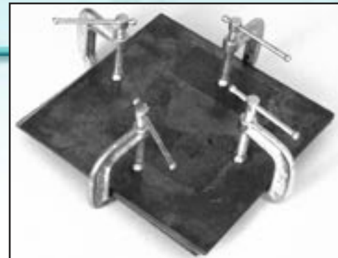
The MEA is clamped between the plates.
