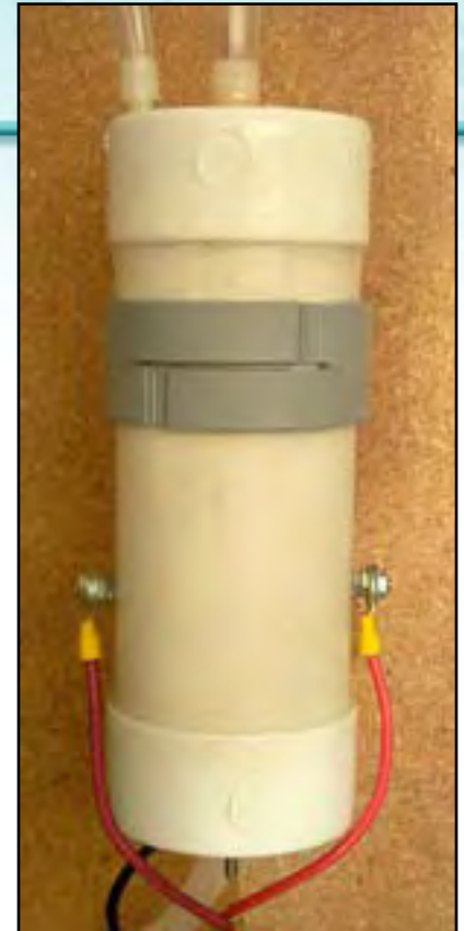
Electrolyzer designed for use with solar panels
