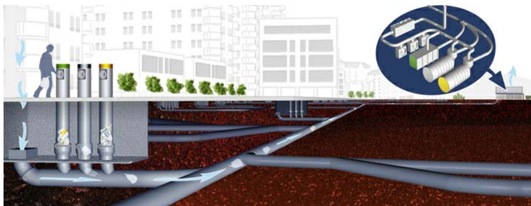
Figure 8.3 The AVAC system (Source http://www.envacgroup.com/ )
