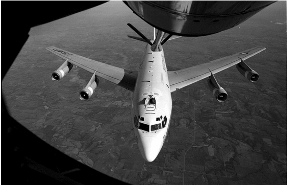
WC-135 , the remaining U.S. aircraft used to gather the airborne particles produced by nuclear testing. U.S. AIR FORCE
