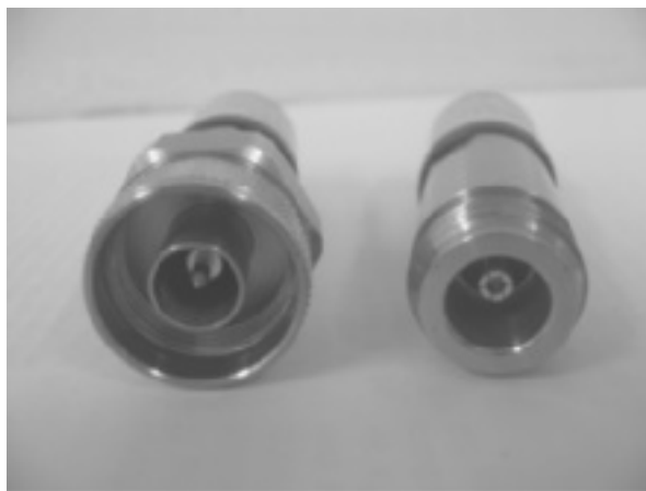
Figure 2.33 Male (left) and female (right) N-type connectors
