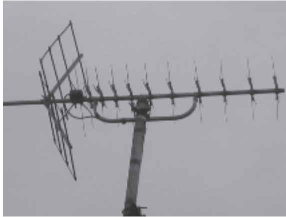
Figure 5.18 A Yagi–Uda TV reception antenna
