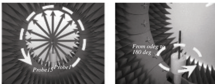
Figure 7.18 Electronic scanning for elevation sampling and AUT rotation for azimuth sampling. [Reproduced by permission of SATIMO]
