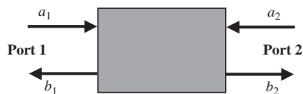
Figure 7.1 A two-port network
