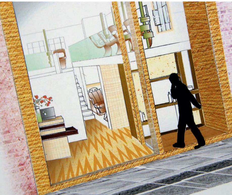
A perspective drawing is used to look inside the building and at the same time show the revised facade that was part of the brief. Both the pattern and scale of the decorative scheme has been hinted at in the rendering, accomplished using Photoshop.
