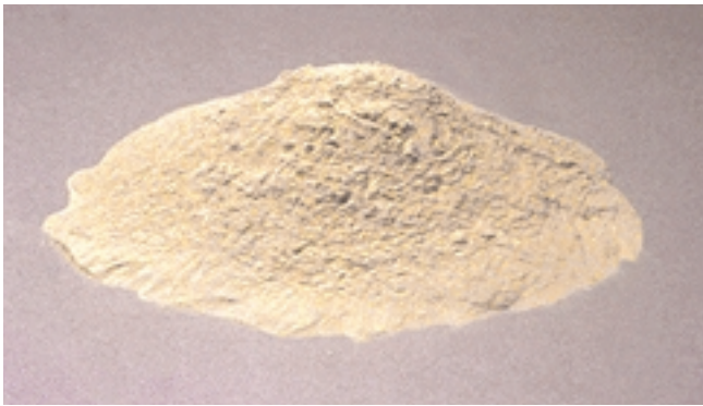
Fig. 3-3. Fly ash, a powder resembling cement, has been used in concrete since the 1930s. (69799)
