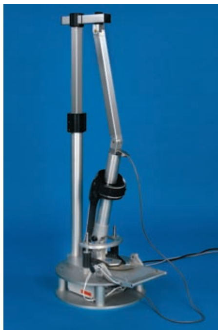
Fig. 4.2.10 Biarticular Reciprocating Universal Compliance Estimator (BRUCE). This comprehensive device includes an adjustable mechanical analog of the full leg and foot. It is manually driven to simulate both dorsiflexion and toe flexion. In this figure a carbon fiber ankle-foot orthosis (AFO) is mounted for testing. A wide range of AFO and footplate sizes can be accommodated. The orthosis can be secured with or without shoes. Forces and moments are monitored continuously to determine the dynamic material and structural properties.
