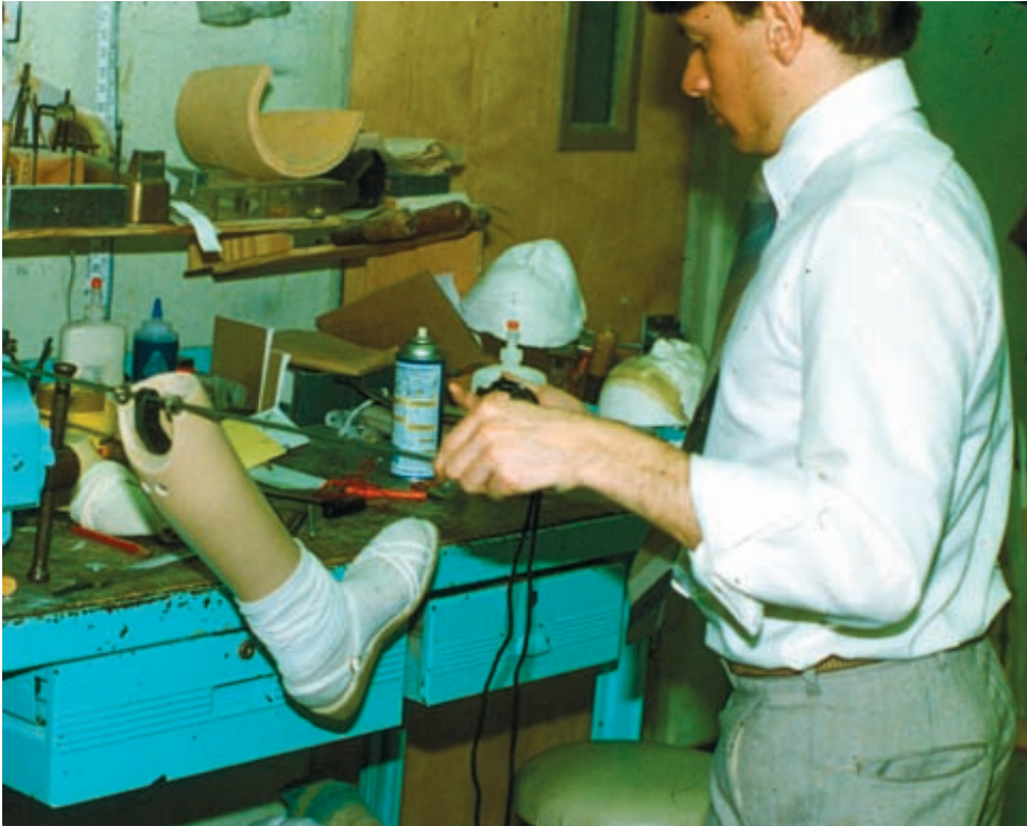
Fig. 1.3.13 A simple experiment that can be done using an above-knee prosthesis with a single-axis knee. The leg acts like a pendulum and its period is dictated by its mass moment of inertia. Since the lower-extremity functions as a compound pendulum in gait, the period of the pendulum (in this case the shank) will be equal to the cadence of the individual to whom it belongs. Given that the cadence of swing is usually found to be much lower than normal in these experiments, a strong argument could be made to bring the mass moment of inertia closer to the fulcrum by minimizing the weight distally and/or adding weight proximally.
