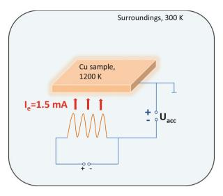
Fig. 9.4 Principle of electron impact heating.  $U_{\rm acc}$  is the high voltage, by which emitted electrons are accelerated toward the copper sample
