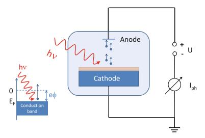
**Fig. 9.5** Experimental setup to measure the photoelectric effect from cathode materials. The *inset* on the *left* illustrates the photo effect in the energy band model of a metal. The work function  $e\phi$  is the difference in energy of the Fermi energy  $E_F$  and the vacuum potential level
