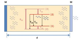
Fig. 10.26 Principle of laser operation (schematic). The active medium is represented by a four-level quantum system within a resonator of d in length. The laser transition is between levels  $|2\rangle$  and  $|1\rangle$ . At least one of the mirrors (M) has nonzero transmission
