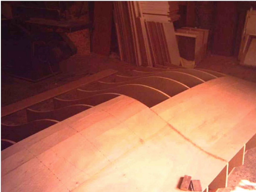
Fig. 11.18 Model production of Solaris Erke solar car for moulding
