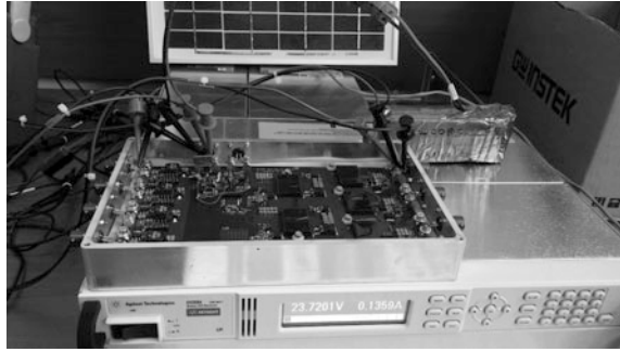
Fig. 18.21 Power module testing conditions
