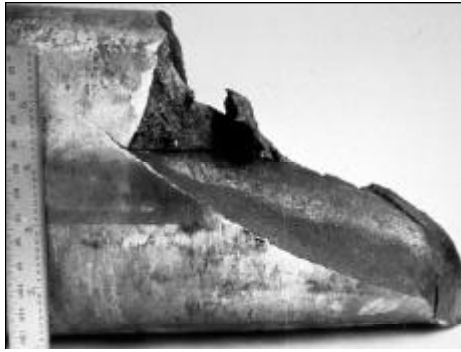
Figure 1. A fatigue failure surface
