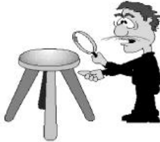
Figure 17. A 'Damage-Tolerant' stool. The stool has some built in redundancy and is inspected regularly
