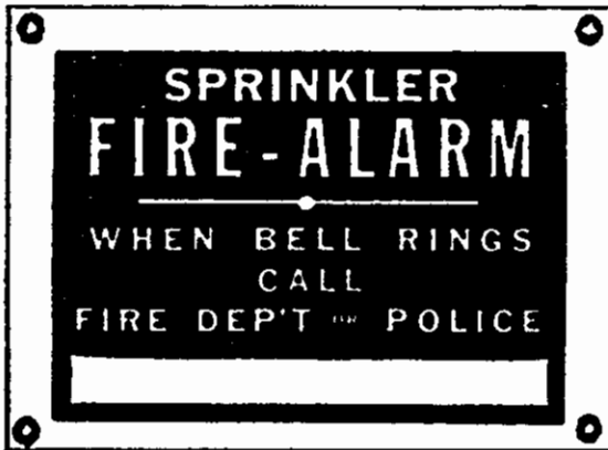
Figure A-4-6.1.1 Identification sign.
