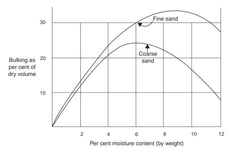
Fig. 19.4. Bulking of sand according to moisture content
