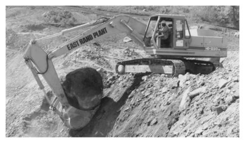
**Plate 3b.** A Kato 162 kW tracked excavator, with  $1.6 \text{ m}^3$  bucket. ACP Holdings, Leicester, UK
