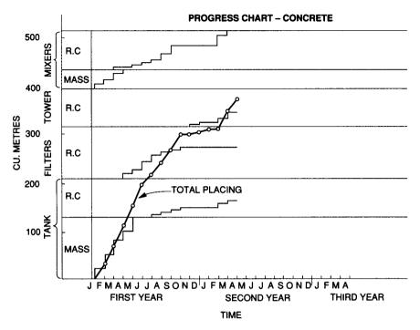
Fig. 14.4. A progress chart for concrete work
