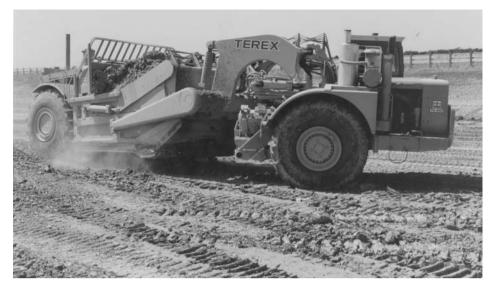
**Plate 3a.** A Terex TS24C 552 kW twin-engined 36 m<sup>3</sup> capacity scraper for earth-moving. Terex Equipment Ltd, Motherwell, Scotland
