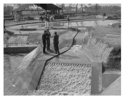
Plate 1a. The hydraulic model for the Ghazi Barotha Hydropower project, Pakistan, 1994
