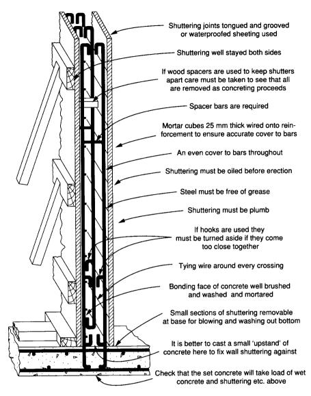
Fig. 19.5. Points to watch in erecting shuttering and reinforcement
