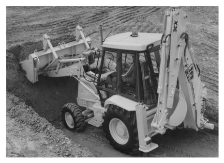
**Plate 8b**. The ubiquitous backhoe loader used on many sites. That shown is the JCB 3CX 56.5 kW, with shovel up to 2.3 m wide and hoe bucket 0.3–0.9 m wide. JCB Ltd, Rocester, UK
