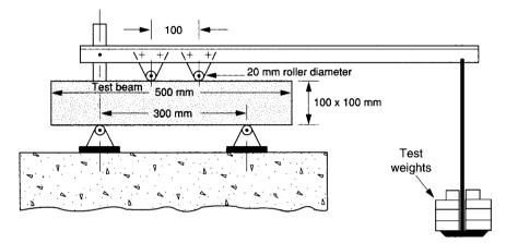
**Fig. 19.1.** Flexural test as BS 1881 on concrete beam for 20 mm maximum aggregate size. For simple site testing (see text) it may suffice to use a single central roller to apply the load
