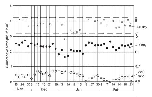
**Fig. 19.2.** Graphical check on concrete test results. A, upper action line 4200 lb/in<sup>2</sup> (29.0 N/mm<sup>2</sup>); B, upper warning line 4000 lb/in<sup>2</sup> (27.6 N/mm<sup>2</sup>); C, lower warning line 3200 lb/in<sup>2</sup> (20.0 N/mm<sup>2</sup>); D, lower action line 3000 lb/in<sup>2</sup> (20.7 N/mm<sup>2</sup>); E, 7 day warning line 2000 lb/in<sup>2</sup> (13.8 N/mm<sup>2</sup>). Each point mean value of five test results.
