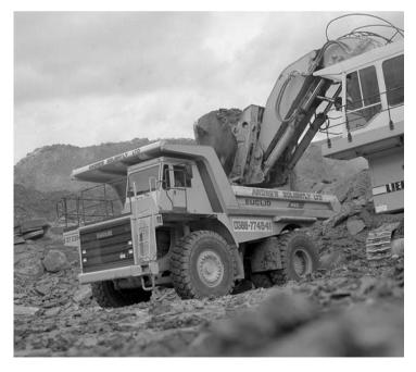
**Plate 2b.** A Euclid R60 522 kW dump truck, 36 m<sup>3</sup> heaped capacity. VME Construction Equipment GB Ltd, Duxford, Cambridge, UK
