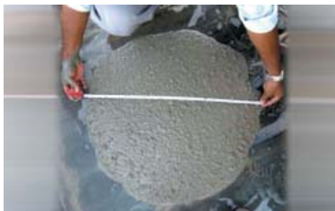
Such a flow is the result of the use of Superplasticizer
