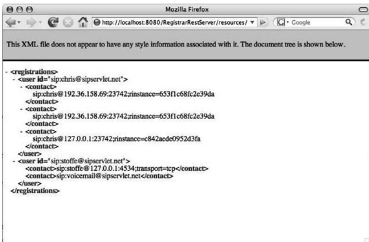
Figure 9.11 Listing after running “curl.” User “Stoffe” has a new contact field.
