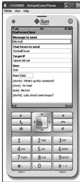
Figure 9.17 WTK Java ME test client running chat application.
