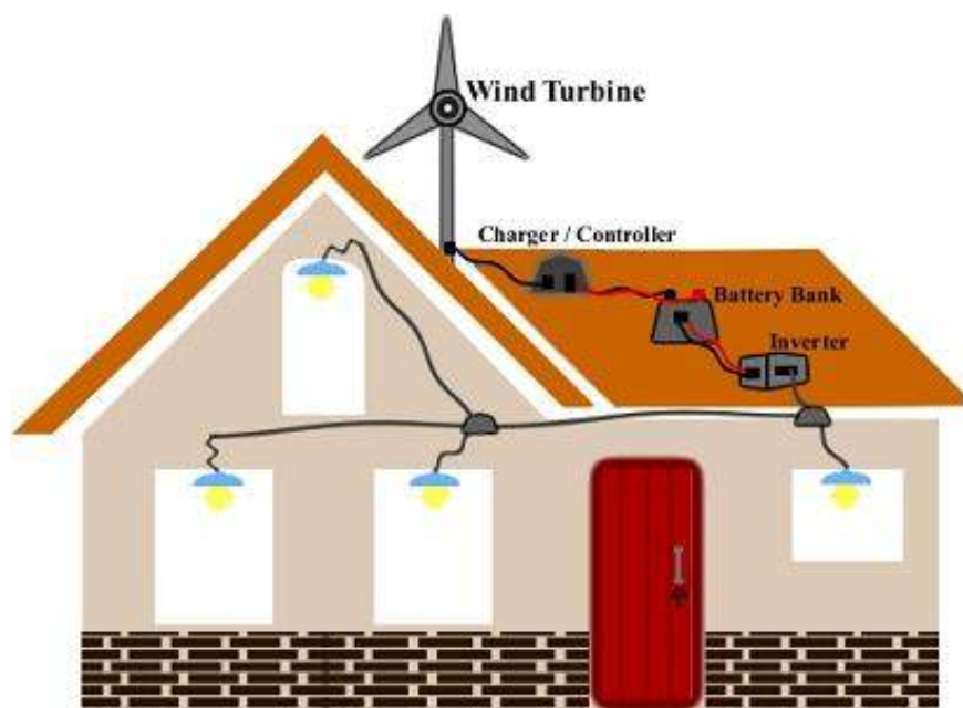
Figure 4.3 Wind Energy System
