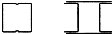
c) Closed built-up sections
