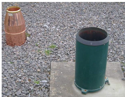
Figure 2 A nonrecording gauge (left) and a recoding gauge (tipping bucket) used in the UK
