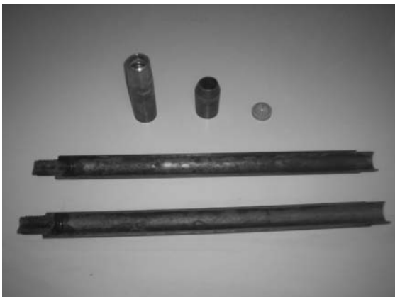
Figure 2.16 (a) Unassembled split-spoon sampler; (b) after sampling (Courtesy of Professional Service Industries, Inc. (PSI), Waukesha, Wisconsin)
