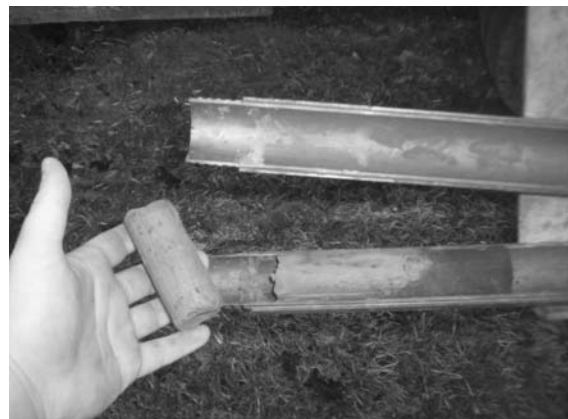
Figure 2.16 (a) Unassembled split-spoon sampler; (b) after sampling (Courtesy of Professional Service Industries, Inc. (PSI), Waukesha, Wisconsin)
