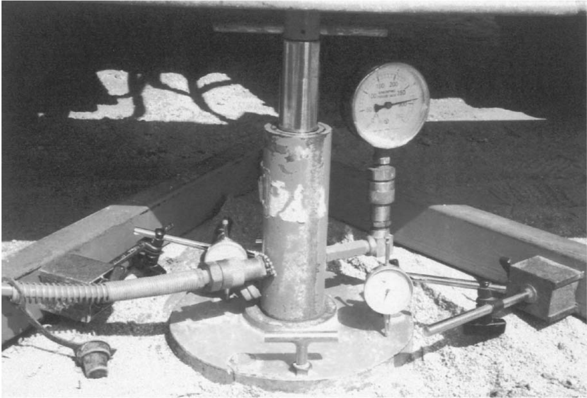
Figure 5.35 Plate load test in the field (Courtesy of Braja M. Das, Henderson, NV)
