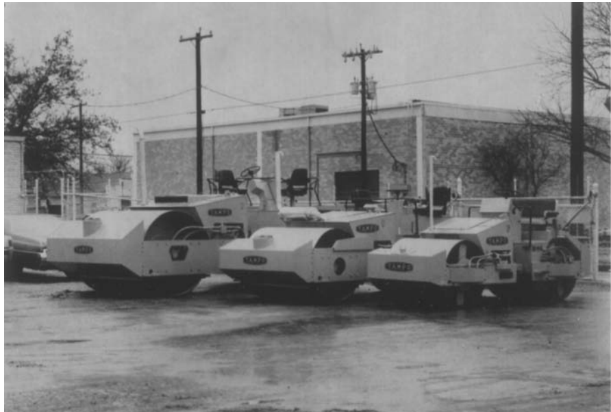
Figure 14.2 Vibratory smooth-wheel rollers (Courtesy of Tampro Manufacturing Co., Inc., San Antonio, Texas)
