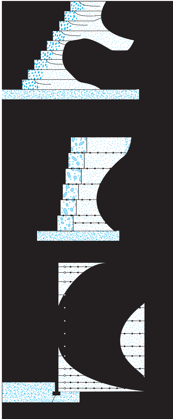
Figure 8.38 Typical schematic diagrams of retaining walls with geogrid reinforcement: (a) geogrid wraparound wall; (b) wall with gabion facing; (c) concrete panel-faced wall (After The Tensar Corporation, 1986)
