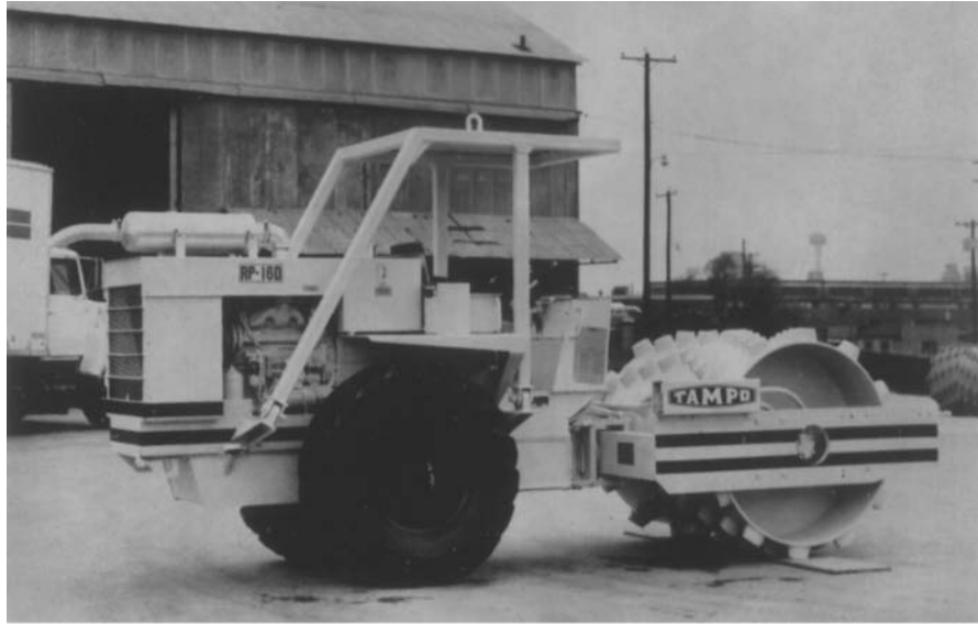
Figure 14.4 Vibratory sheepsfoot roller (Courtesy of Tampro Manufacturing Co., Inc., San Antonio, Texas)
