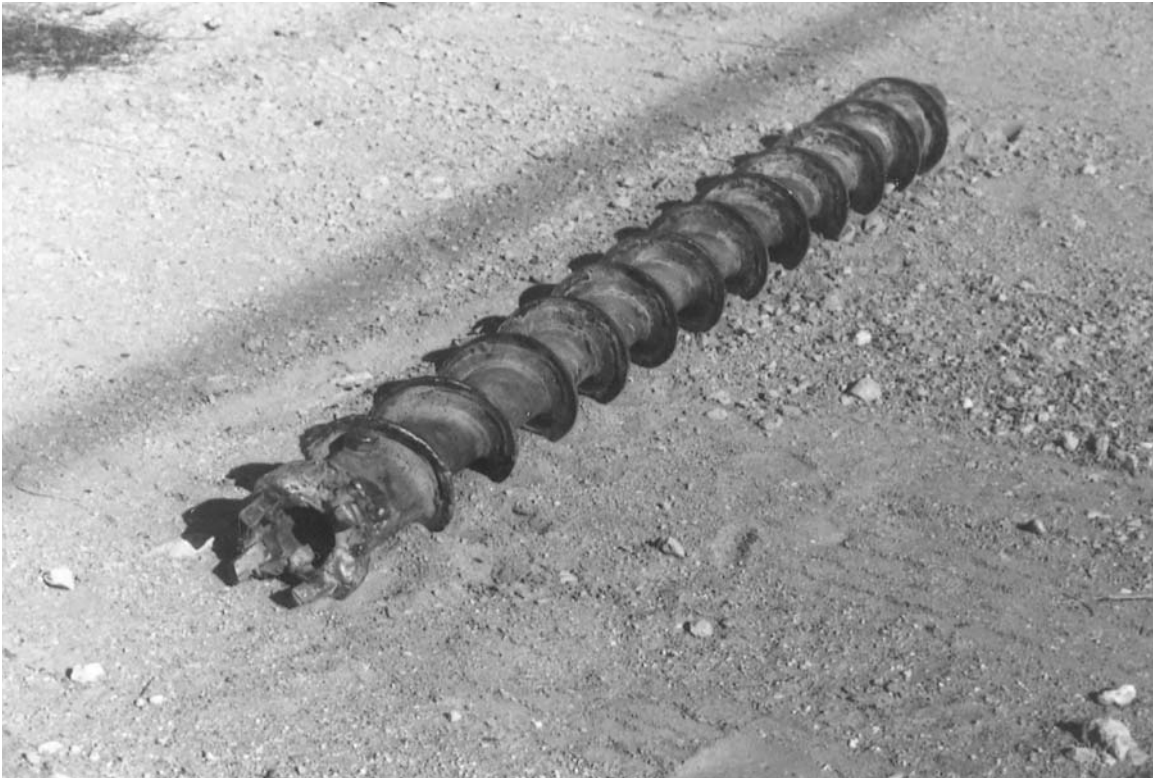
Figure 2.11 Carbide-tipped cutting head on auger flight (Courtesy of Braja M. Das, Henderson, NV)
