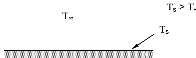
Figure 3-12 Natural convection over a horizontal flat plate
