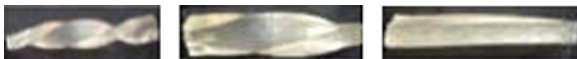
Fig. 6.3 Photo series demonstrating the shape memory effect of a polymer network from a temporary shape to a permanent shape at 25°C after twisting and freezing at -20^{\circ}\text{C} (from left to right)
