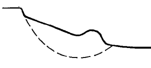
40.12 The same slope after failure. Note 'hump' at bottom of slip
