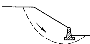
40.13 The use of a retaining wall at the toe of a slope does not prevent a slip circle failure
