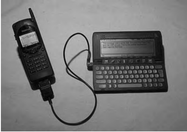
Figure 6.8 A GSM phone connected to a palmtop.
