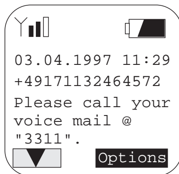
Figure 6.7 Display of a mobile station with a mobile-terminated short message.
