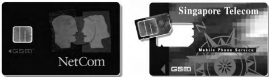
Figure 8.1 Two different sizes of SIM cards are available (courtesy of Schlumberger).
