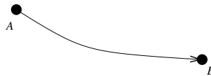
FIGURE 3.10: Global orientation of mesh edges based on a unique enumeration of vertices (here index(A) < index(B) ).
