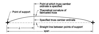
Taking L as the distance from the point at which truss camber is specified to the closer point of support, in. [mm], the tolerance on truss camber at that point is calculated as L/800. L must be equal to or less than one-half the span.
