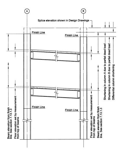
Figure C-7.1. Effects of differential column shortening.
