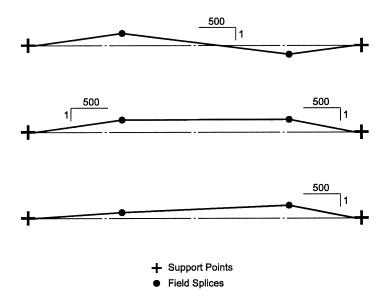
Figure C-7.7. Alignment tolerances for members with field splices.
