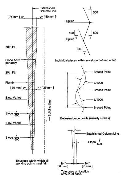
Note: The plumb line through the base working point for an individual column is not necessarily the precise plan location because Sect. 7.13.1.1 deals only with plumbness tolerances and does not include inaccuracies in location of the Established Column Line, foundations and anchor rods beyond the Erector's control
