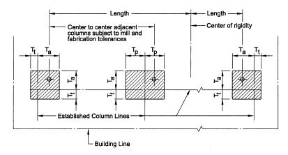
Figure C-7.2. Tolerances in plan location of column.
