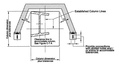
If facia joints are set from nearest column finish line, allow ±5/8 in. [16mm] for vertical adjustment. The entity responsible for the facia details must allow for progressive shortening of steel columns.
